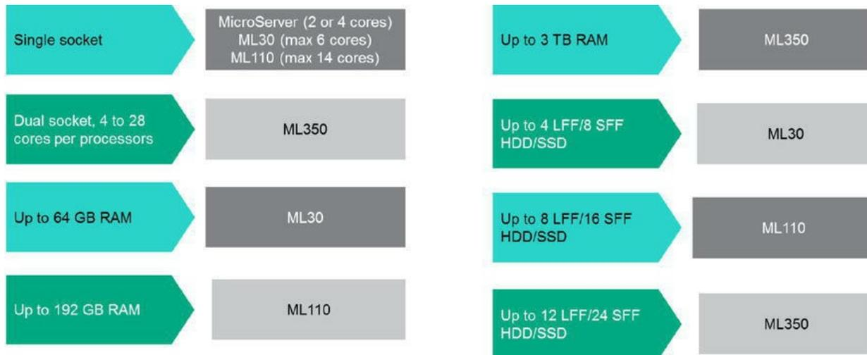
Figure 2-6 Selecting an HPE ML server platform, based on performance, memory, and storage requirements
