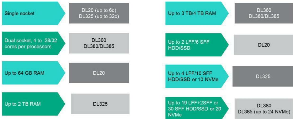
Figure 2-49 Selecting an HPE DL server platform, based on performance, memory, and storage requirements
