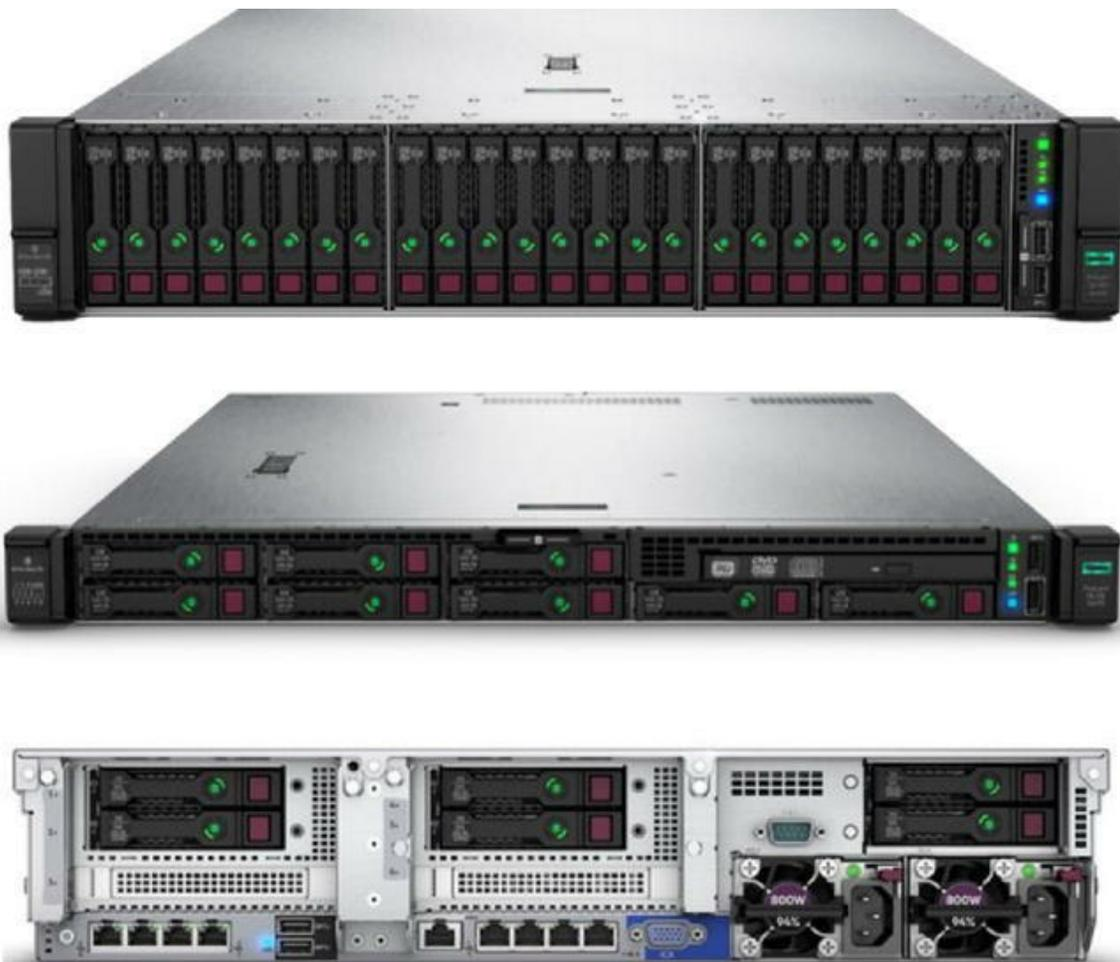
Figure 2-51 HPE ProLiant Gen10 rack servers are based on industry-standard x86 architectures
