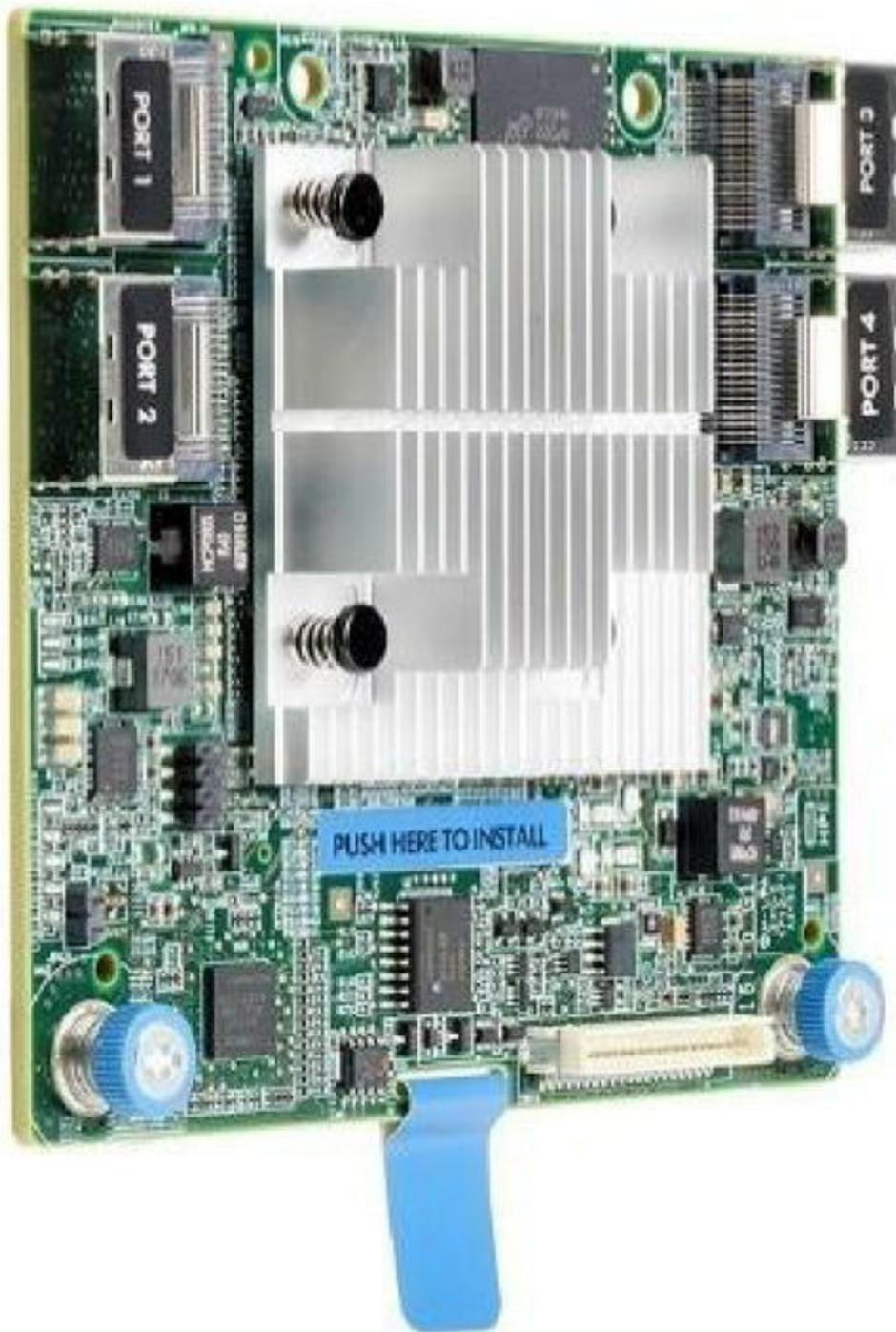
Figure 2-28 HPE Smart Array Controller
