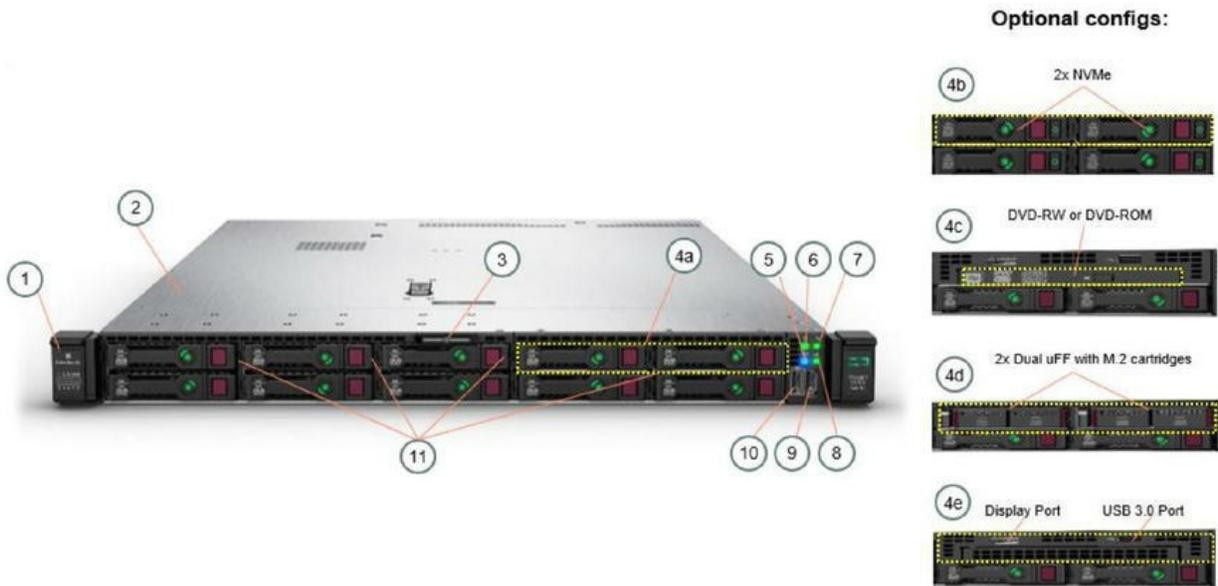
Figure 2-57 ProLiant DL360 Gen10 Server with eight LFF, front view
